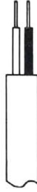
Blue to N (Neutral) or Black Brown to L (Live) or Red
